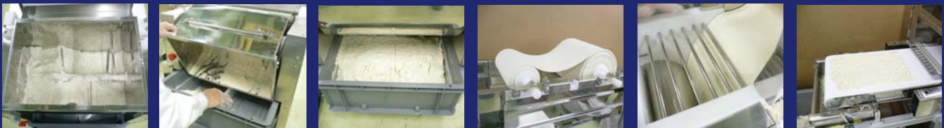
1) Put flour and water. 2) Place a container. 3) Make dough. 4) Make flat. 5) Cutting. 6) Complete.
